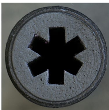
Figure 3: Fuel grain cross section
