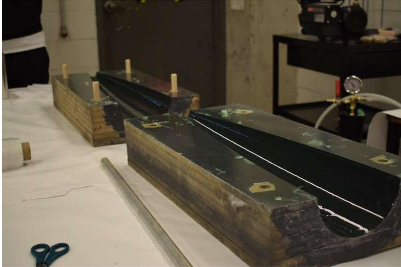
**Fig. 35** Nosecone Mold Halves
