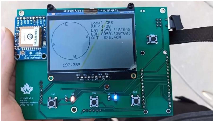
**Fig. 142 ST PATS local GPS and compass test**
