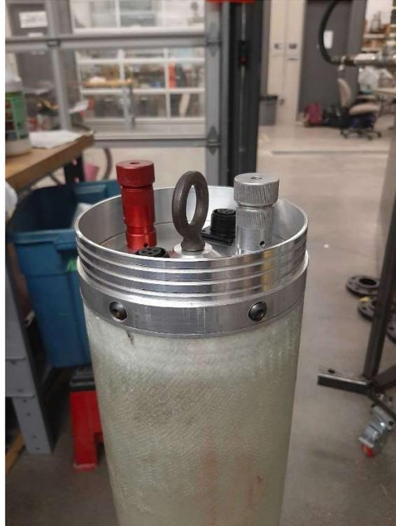
**Fig. 43 Recovery Bulkhead CouplersPayload Bay**
