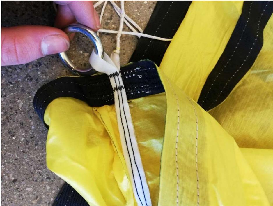
**Fig. 87 Rings at the inner seam line of each gore for routing**
