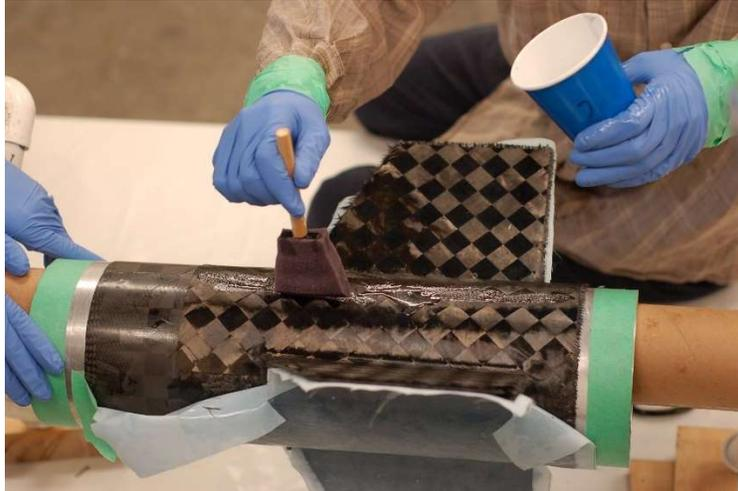
**Fig. 56 Wet Hand-Layup Vacuum Bag Consolidation**
