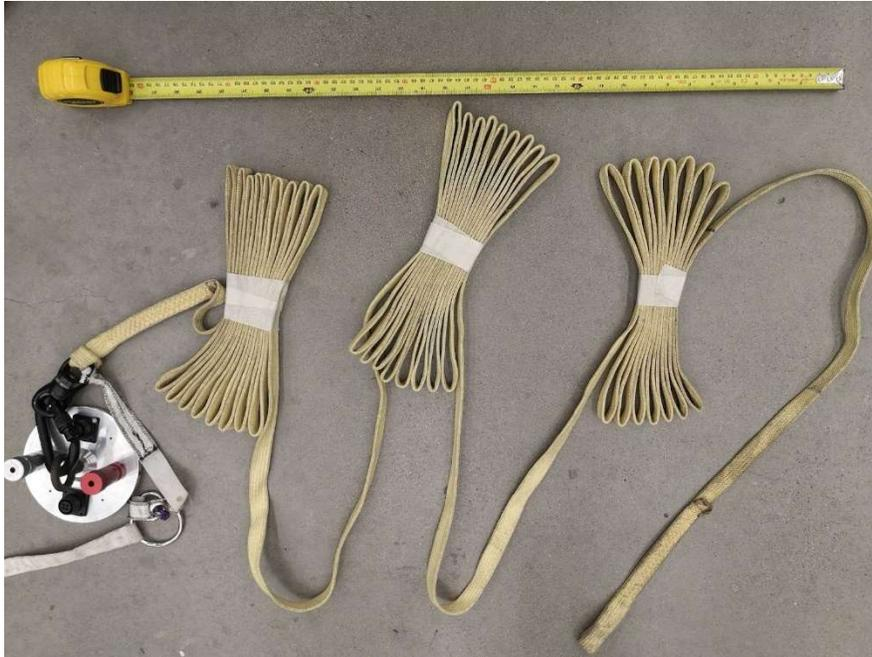
**Fig. 75 Partially rigged shock cord**
