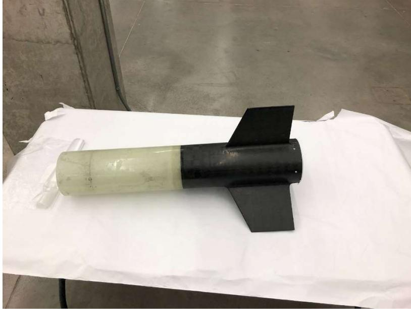
**Fig. 58** Fin Can bonded to the CC Bodytube
