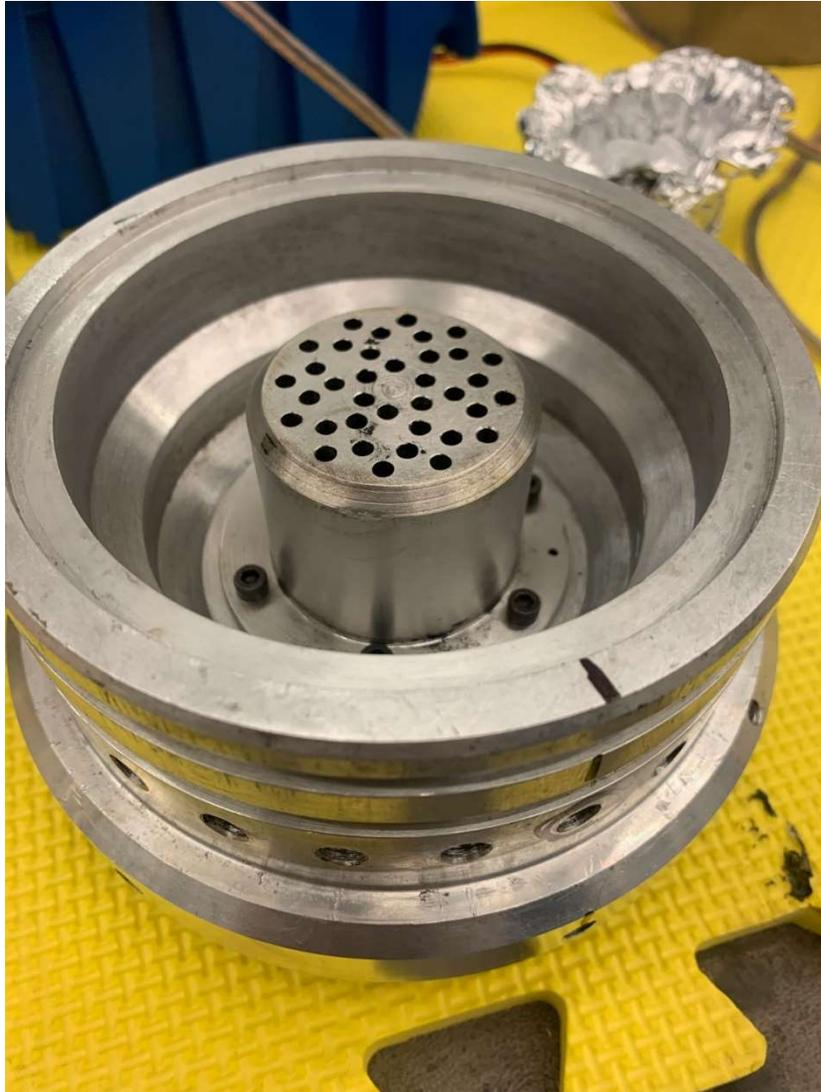
**Fig. 15 36-element showerhead injector installed in injector bulkhead**
