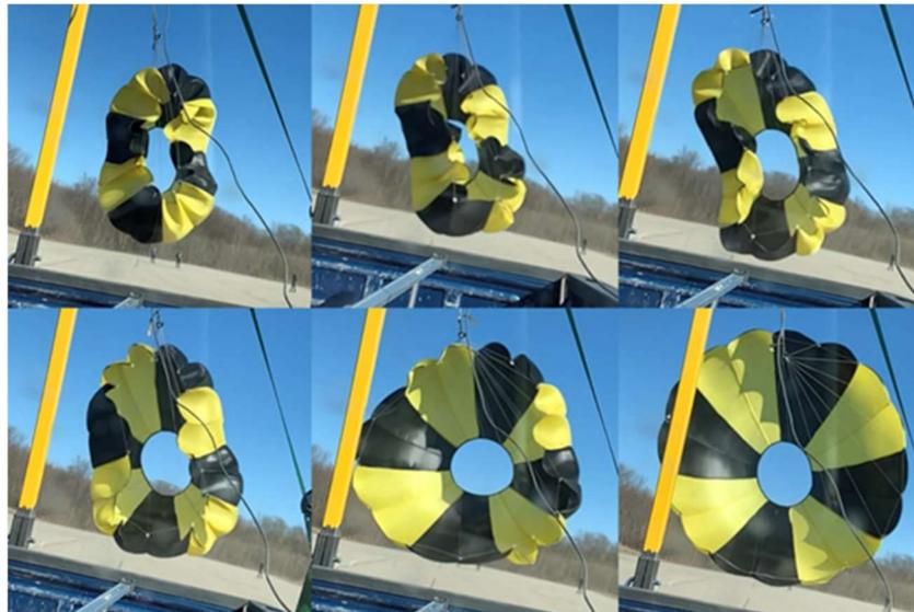
**Figure 8 Disreefing sequence on the full-scale parachute.**
