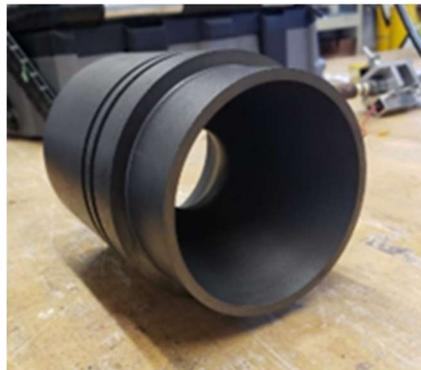
**Fig. 23 The as-machined graphite ‘bell’ nozzle**
