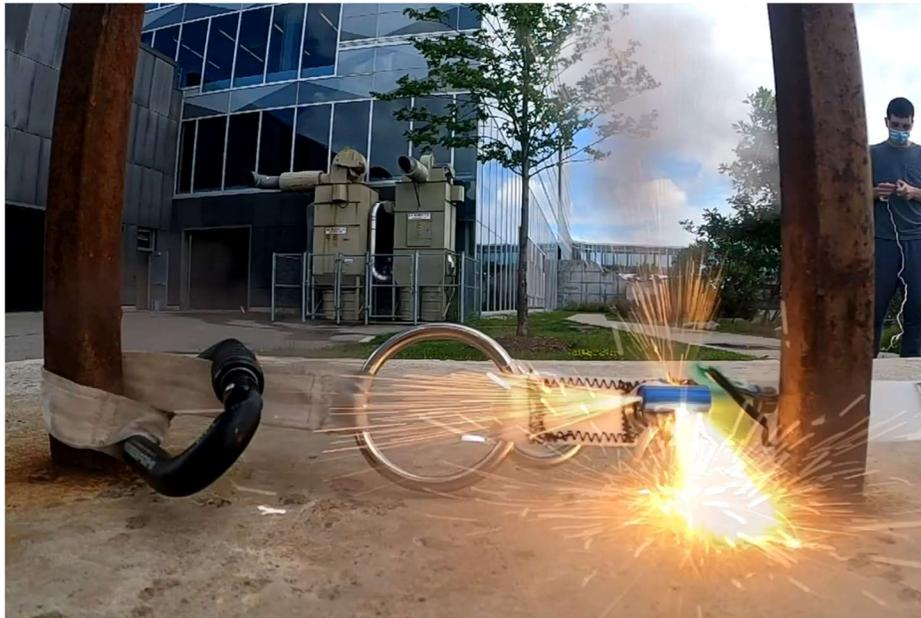
**Figure 14 Two ring release undergoing testing**
