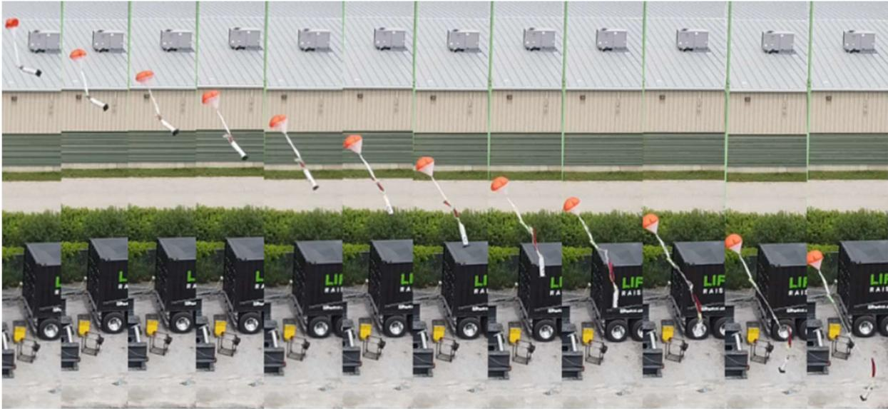
**Figure 10 Pilot Parachute test drop from 60 ft test tower**
