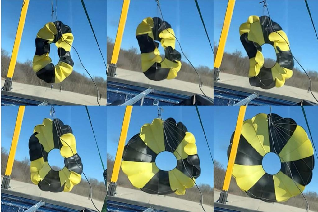
**Fig. 67 Disreefing sequence of the parachute during a 2021 truck test**
