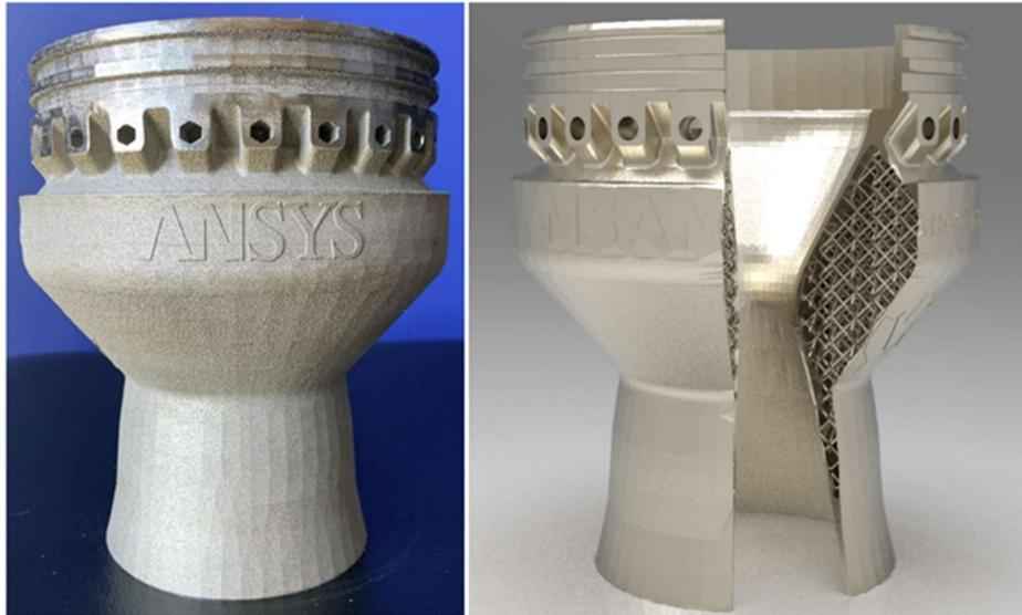
**Fig. 17 A cross-sectional render of the design (left) and the actual printed part (right)**
