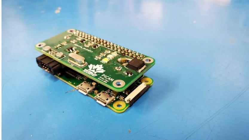
**Fig. 112 PiCam board attached to a Raspberry Pi Zero**
