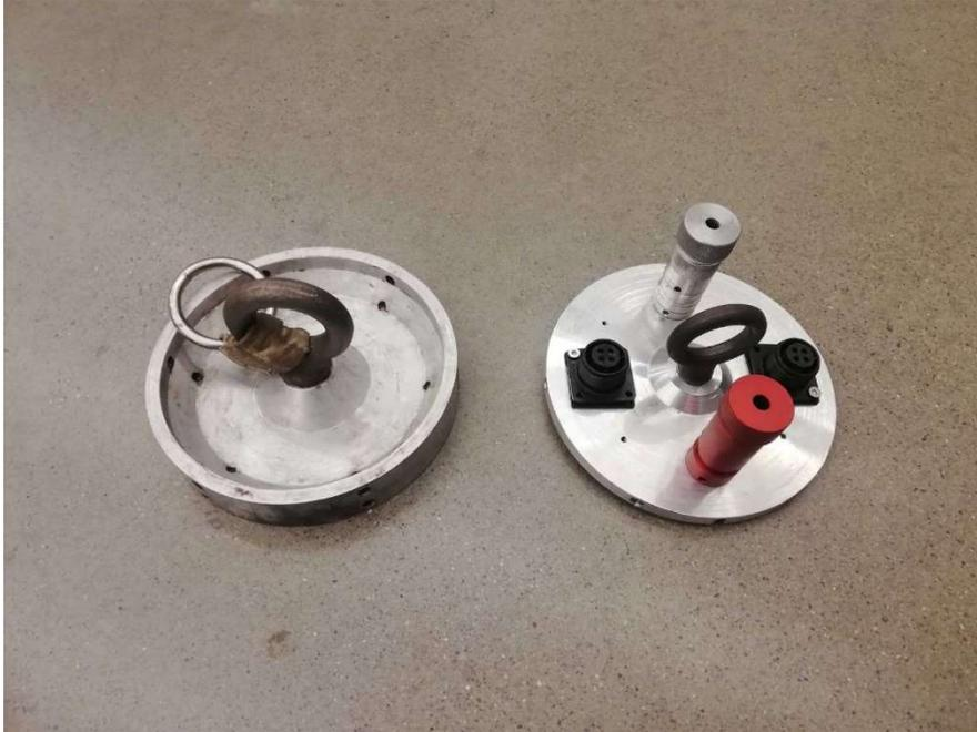
**Fig. 76 Old parachute bulkhead on the left (2019), new parachute bulkhead on the right (2022)**
