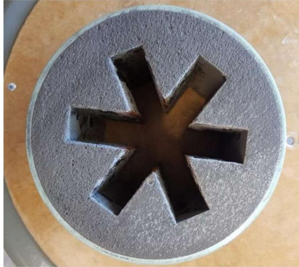
**Fig. 8 Cross-section of Kismet fuel grain [1]**
