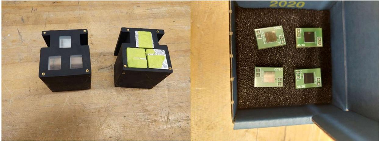
**Fig. 148 Scintillators and enclosures (left) SiPMs (right)**
