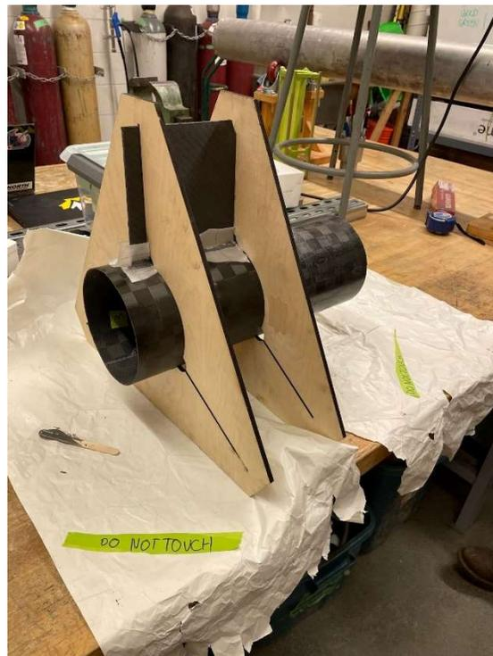
**Fig. 55 Bonding Fins Onto Fin Can Bodytube**
