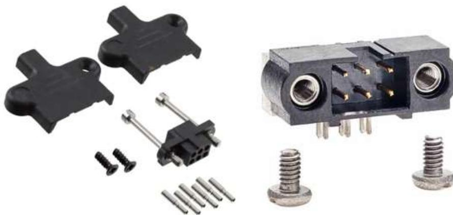
**Fig. 99 Female Harwin Datamate connector assembly (M80-9410642) with a Male Harwin Datamate PCB mounted connector (M80-5400642) beside it**
