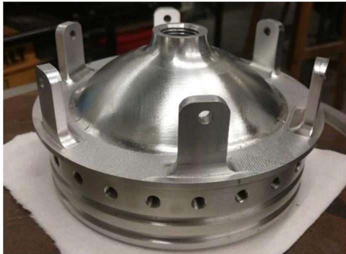
**Fig. 10 Hemispherical oxidizer bulkhead [1]**
