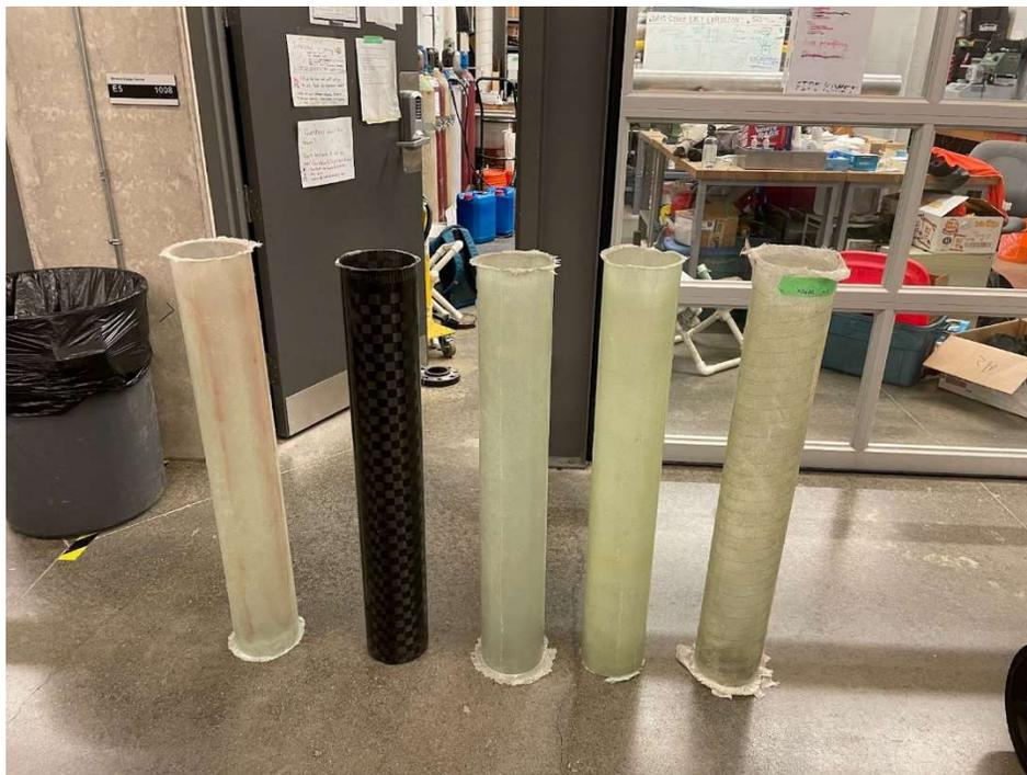
**Fig. 40 Fiberglass and Carbon Fiber Bodytubes Fabricated Using VARTM**
