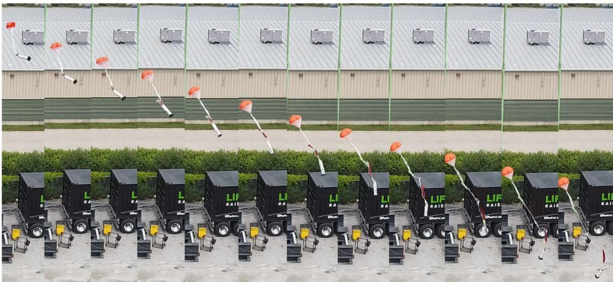
**Fig. 73** 60 ft Drop test, conducted at the LiftWerx Test Tower, to characterize the height required to deploy the parachute from its bag
