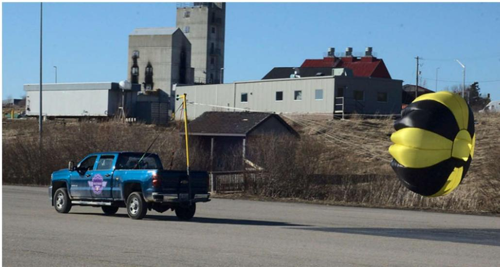
**Figure 7 truck testing with the full scale parachute.**
