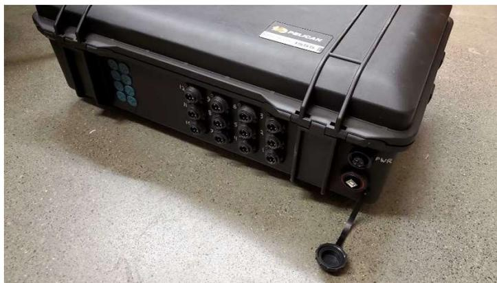
**Fig. 138 Connector ports on DAQ system**
