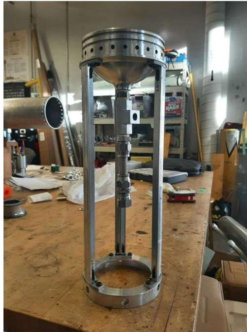
Figure Oxidiser Tank Aft Skirt
