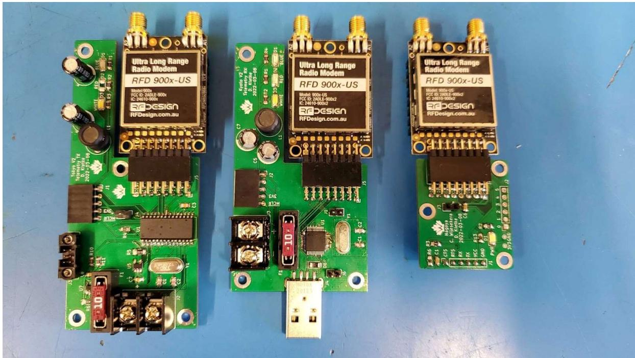
**Fig. 125 Live telemetry transmitter, receiver and breakout**
