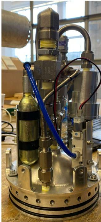
**Fig. 25** Assembled vent section without body tube
