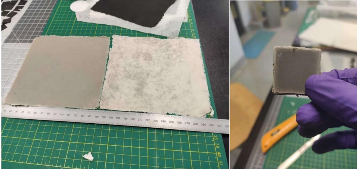
**Fig. 150 BNNT TPU sheet cut and pressed into a final sample**
