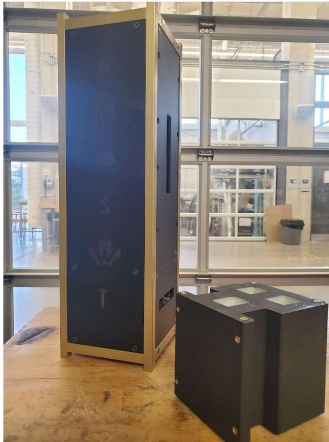
**Fig. 149 Assembled CubeSat displayed along with scintillator enclosure**
