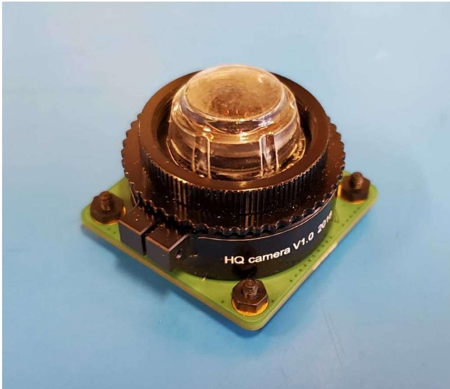
**Fig. 113 PiCam camera module with 180-degree lens attached (protective cover installed)**
