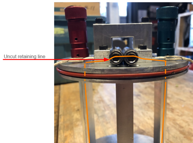
Figure 1.18: Retaining line path through retaining brackets and line cutters.
