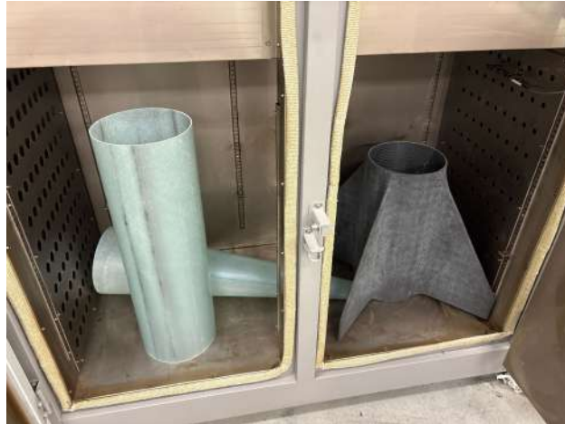
Figure 7.1: Composites in curing oven
