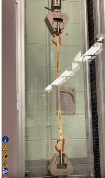
Figure 10.15: Energy modulator tensile test
