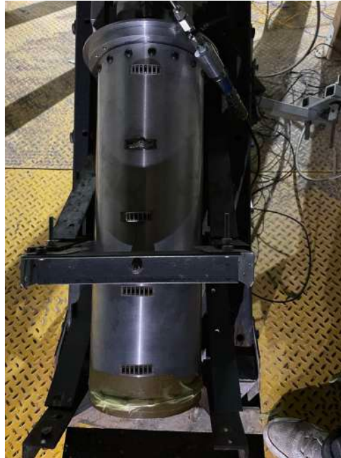
Figure 8.7: Aluminum CC casing after 9s burn
