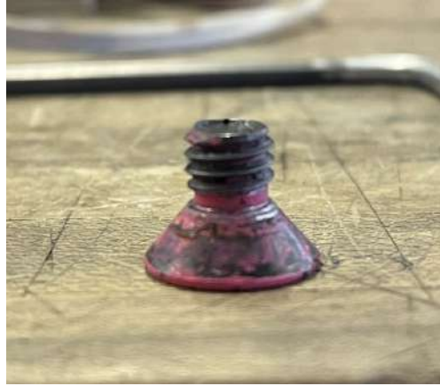
Figure 8.16: Undercut on countersunk tank bolt
