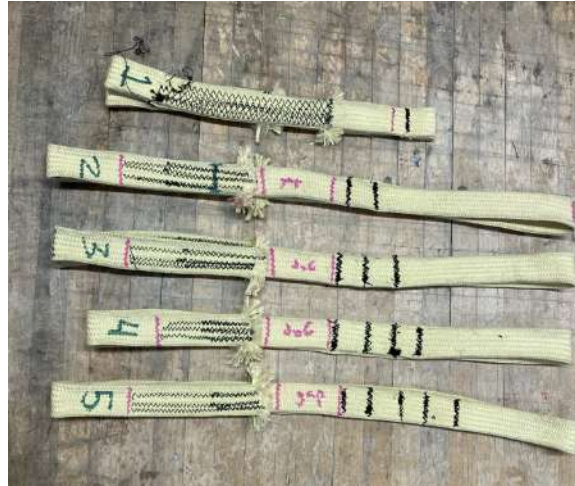
Figure 10.11: Rigging stitching pattern tensile test samples
