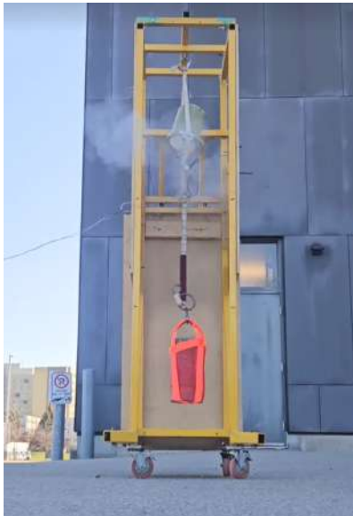
Figure 10.19: Line cutters and 2-ring release testing
