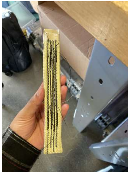
Figure 10.14: Energy modulator stitching pattern prototype
