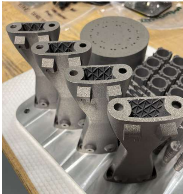
Figure 7.9: Printed longerons on the build plate after de-powdering.
