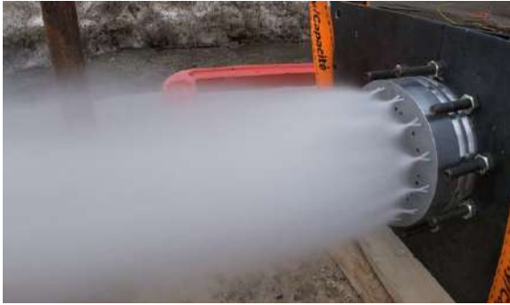
(a) Cold flow testing of the fuel channels using high-pressure water. The two fuel streams of each element impinge, resulting in atomization of the fuel.
