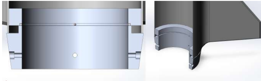
Figure 7.21: Spin can final cross-section
