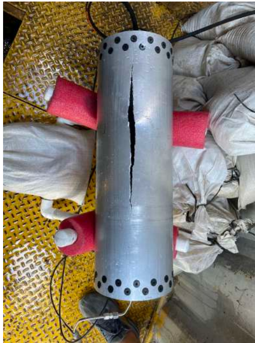
Figure 8.17: Hoop failure of burst test tank
