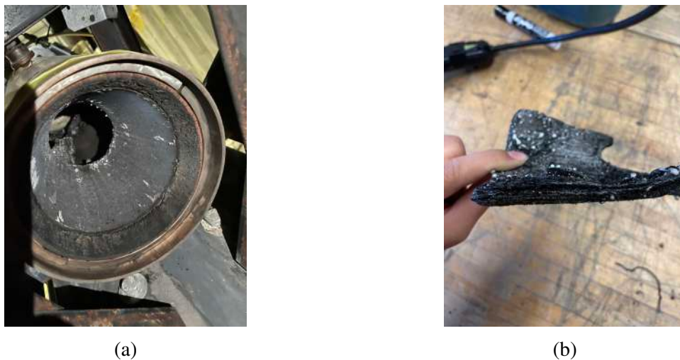
Figure 8.6: (a) Fibreglass beads on nozzle exit post-ELSF5; (b) Char formation in phenolic fibreglass ablative
