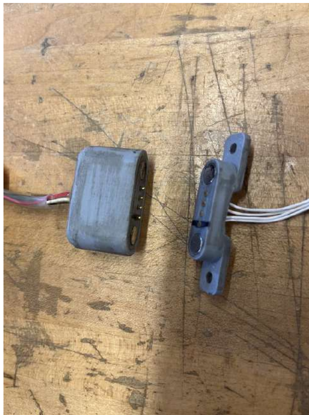
Figure 11.7: Rocket electrical disconnect
