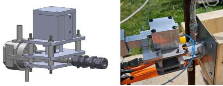
Figure 8.29: Ground-side mechanism and pneumatic actuator in CAD (left) and during tests (right)
