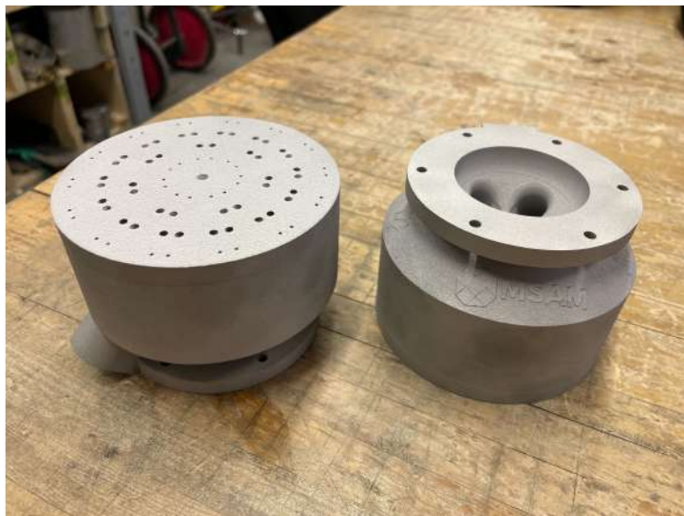
Figure 8.12: Printed injectors after being cut from the build plate but before post-machining.
