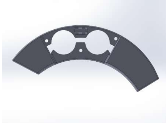
Figure 10.4: Recovery harnessing protector
