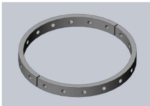
Figure 8.3: Split retaining ring
