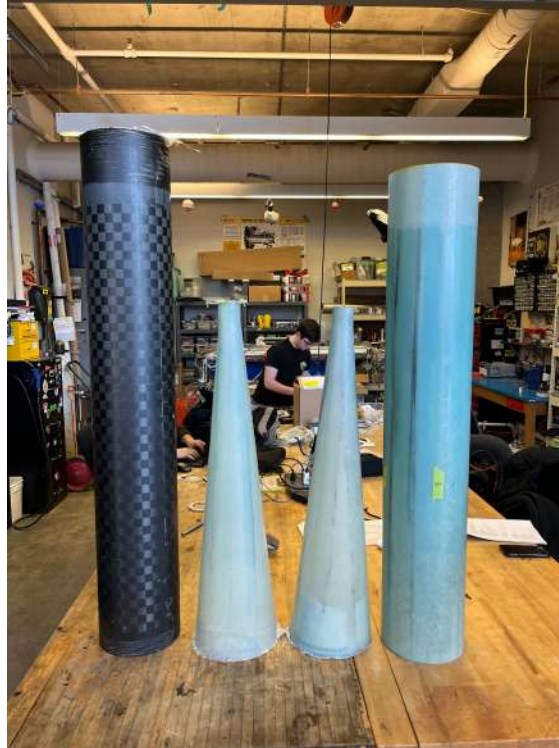
Figure 7.3: SRAD composite parts (from left to right): Fincan tube, nosecones, avionics/parachute bay tube
